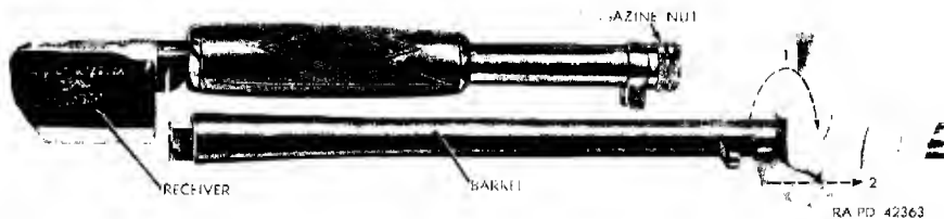
Figure 66—Barrel Disengaged from Receiver—Magazine Nut in Disengaged Position—Ithaca Shotgun M37
